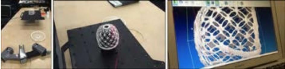
Figure 3. Polhemus Scorpion handheld 3d laser scanner; the scanning process; and the 3D scan.
